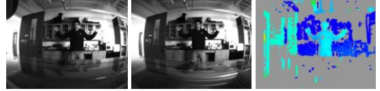
Figure 10: The left and middle images are raw images from the Bumblebee2. The right image is the disparity image generated by the ROS stereo image pipeline
