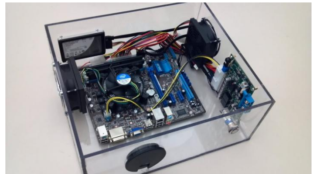
Figure 6: Redblade's computer platform in its housing. This housing can be easily removed from the vehicle if necessary.
